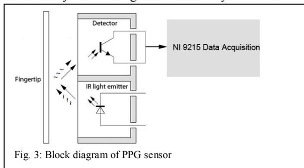
Fig. 3: Block diagram of PPG sensor
